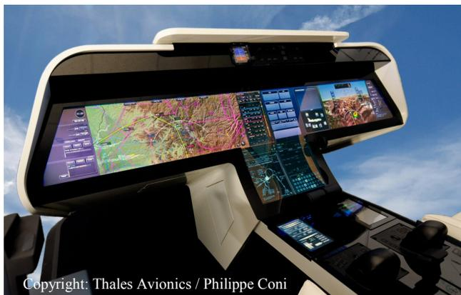
Figure 2. The ODICIS single-screen tactile cockpit.
