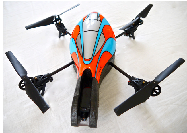
Figure 1. AR.drone ( www.ardrone.com ). The scene ahead is transmitted from the nose camera to a control monitor.
