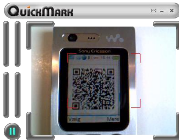
Fig. 5 Decoding a QR-code from a PC webcam: Snapshot of a phone SE W880i displaying a QR code in a Web page.
