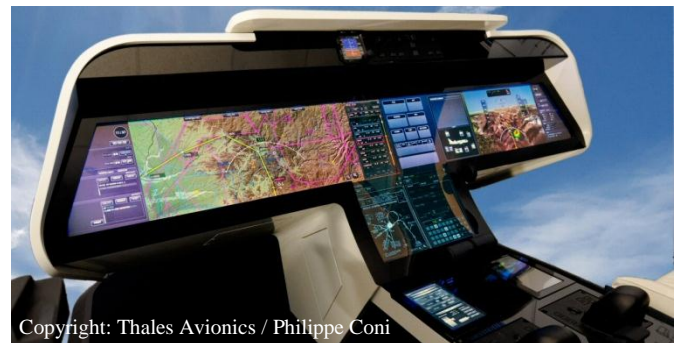
Copyright: Thales Avionics / Philippe Coni Figure 1: The ODICIS large tactile single-screen cockpit
